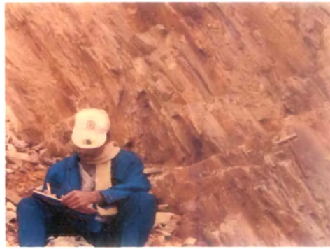
Photo-4.4b: Tabular thin plates or sheets developed due to slaty cleavage in phyllite at Mawryngkneng near petrol pump.
